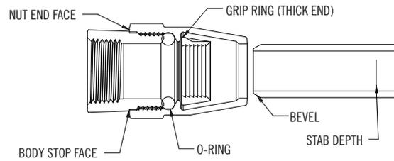
The A.Y. McDonald Series compression system is a simple convenient method of connection for tube size service materials.
