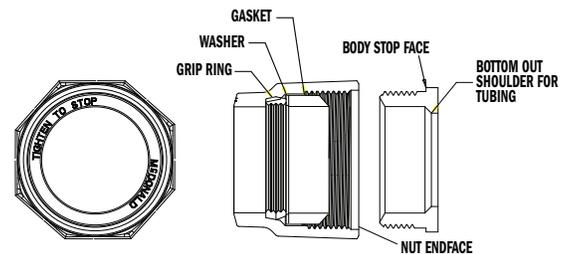
The A.Y. McDonald McGrip "G" & "-3G" Series compression system is a simple convenient method of connection for tube size service materials
