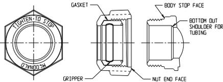
Tighten the CTS McQuik "Q" Series nut or the PEP McQuik "-3Q" nut to the stop. The end face of the nut is to contact the stop face of the body.
